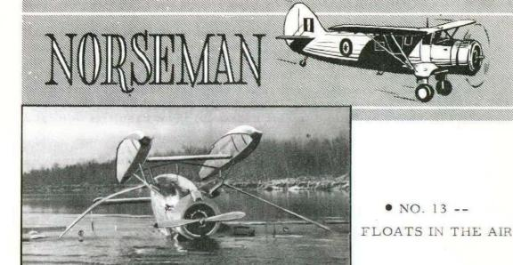
This aircraft was proceeding to a water base for the purpose of changing from floats to wheels. Shortly after touching down (while carrying out a "glassy water" landing) the aircraft struck a sand bar and turned over on its back.
