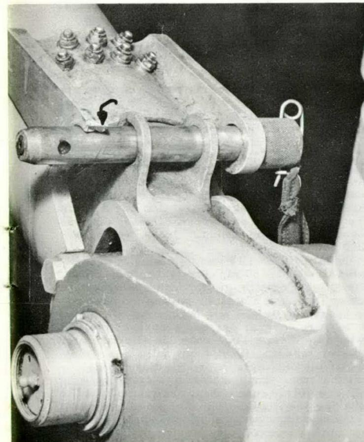
indicated an unsafe condition and the horn sounded. The groundcrew tried to insert the safety pin in the port radius strut but it would pass through only three of the four holes.
