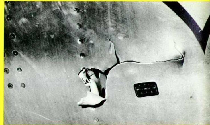
"Over the past 10 years, we have lost two fighters and officially recorded 271 such (ricochet) incidents (156 F-4s). In the past 3-1/2 years, the USAF has spent 1.3 million dollars on aircraft parts alone to repair ricochet damage incurred during routine practice strafing missions".
