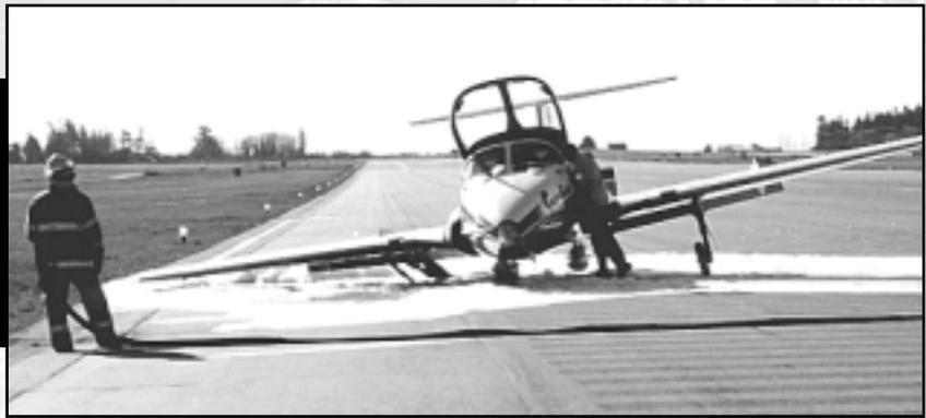
The aircraft was number five of a 9-plane formation landing after an on-field air show practice at 19 Wing Comox. During touchdown on runway 29, the aircraft experienced a firm landing and the right-hand main landing gear and nose-gear collapsed.
