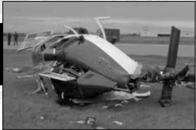
the air, rotated through 720 degrees and impacted the ground 200 feet from the point of initial ground contact. The pilots received minor injuries and the aircraft sustained "A" category damage.
