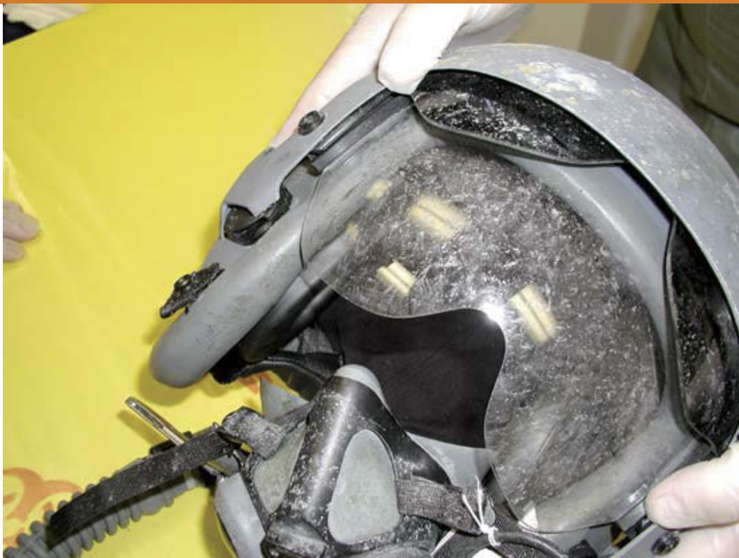
Figure 4. Helmet, visor and mask damage due to MDC and canopy material
