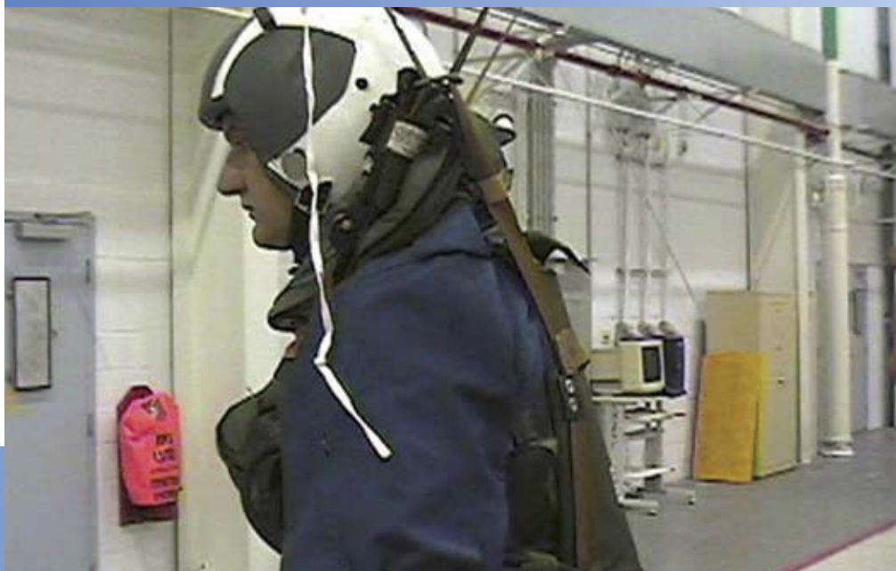
Figure 3. Suspension test showing excessive triangular void above the shoulders
