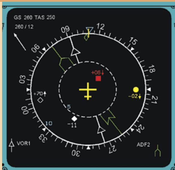
Figure 4. TCAS display on a horizontal situation indicator
