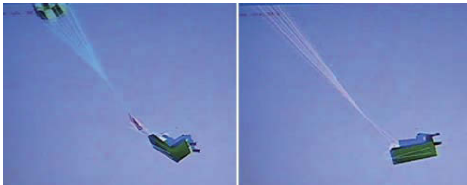
Figure 2. Extraction of main parachute by drogue chute; approximation of misalignment of seat/pilot with main chute axis on inflation
