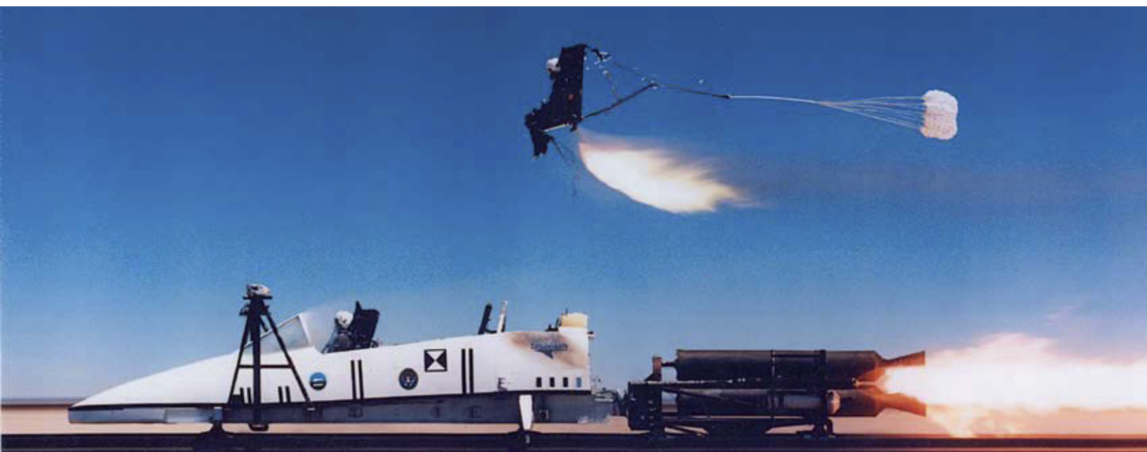
Figure 1a. NACES ejection test showing the multi-point attachment drogue chute
